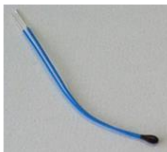
Figure 25 Temperature sensor as thermistor (NTC). (Range -55 to 70°C \pm 0,2 °C)
