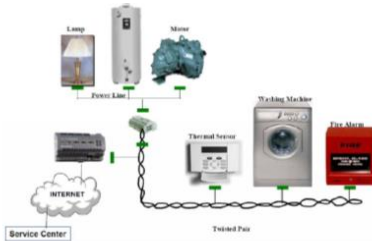
Figure 12 Example of a LonWorks network on twisted pair [6]
