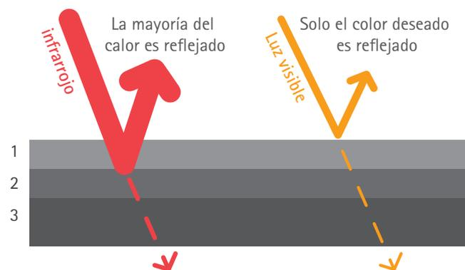
1. COATING ANTI-UV 2. MEMBRANA IMPERMEABLE COOL COLOUR 3. SOPORTE
