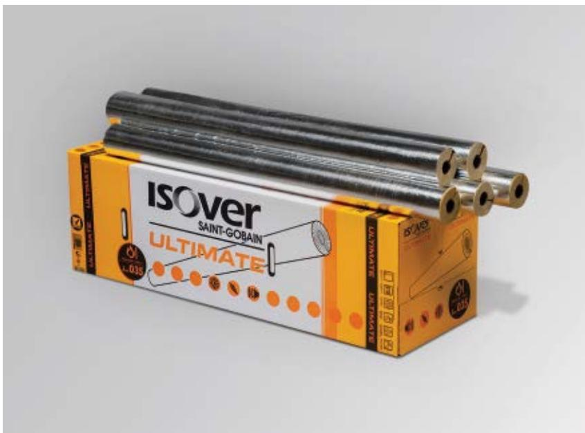
U Protect pipe solutions provides an easy to install and lightweight efficient solution for thermal and acoustic insulation and fire resistance in HVAC pipe systems, using ULTIMATE mineral wool. ISOVER U Protect pipes provides topclass thermal insulation for hot water and heating pipes and secures the building fire safety for penetrations up to EI 120 according to EN 1366-3. Alufacing provides efficient water vapour barrier when intact and seems carefully taped.
